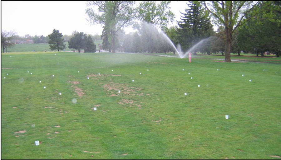
Distribution Uniformity test on #4 fairway.
