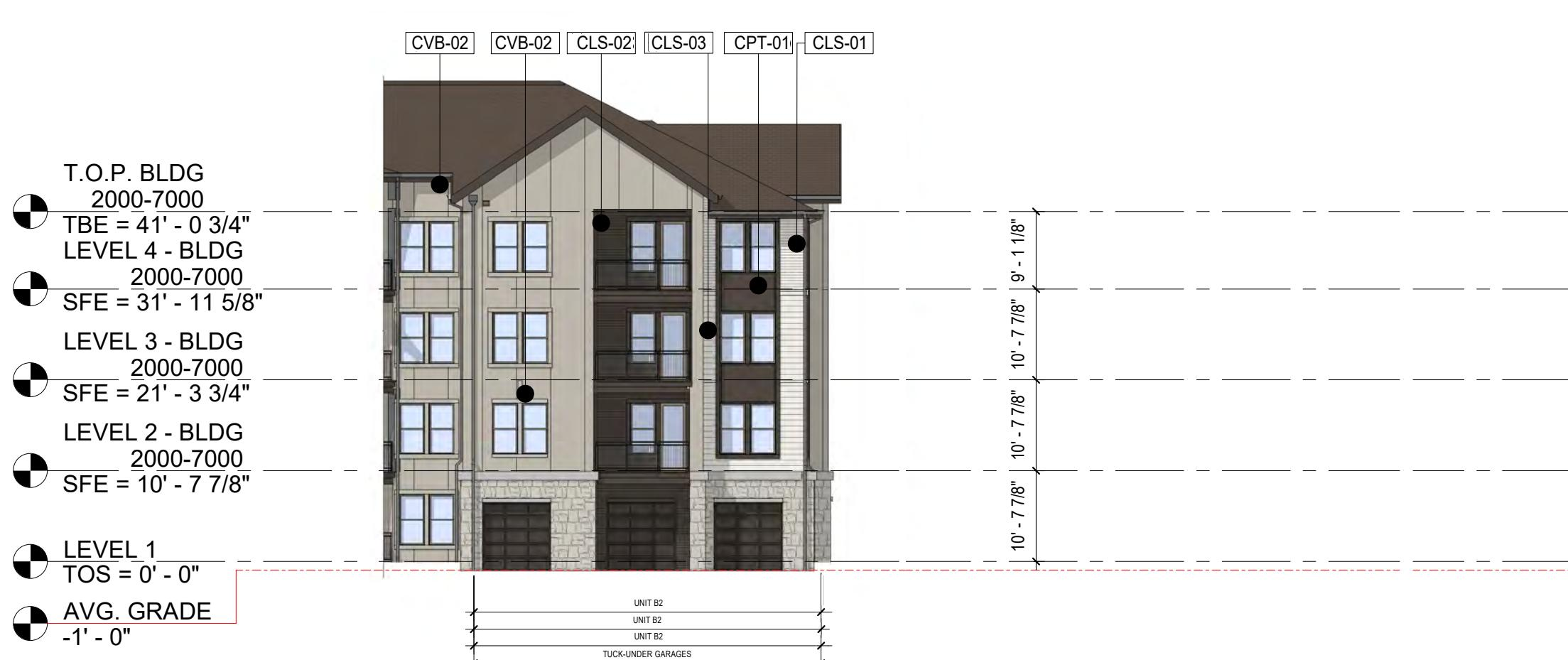
EXTERIOR BUILDING NORTH WEST ELEVATION - TYPE 2 -
