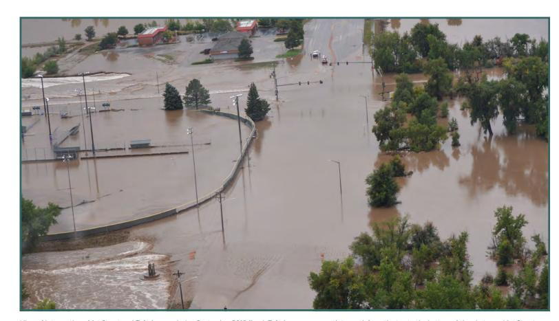
View of intersection of 1st Street and Taft Avenue during September 2013 flood. Taft Avenue runs south to north from the top to the bottom of the photo, and 1st Street runs east to west from left to right. This photo shows overtopping in the intersection and to the north. These overflows spilled into North Jayhawker pond and cascaded through the River's Edge Natural Area. Flow through the Taft Avenue Bridge can be seen in the bottom left corner of the photo.
