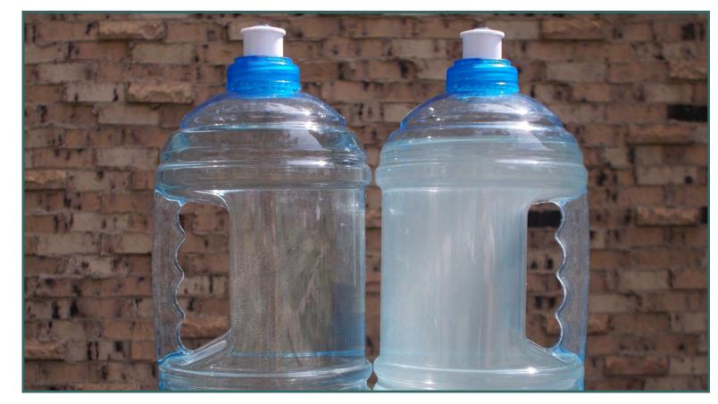
Comparison of sample from Mariano Exchange Ditch with sample from river just upstream of discharge point. The ditch has elevated levels of sediment and is noticeably turbid in comparison with the river upstream. The Consolidated Home Supply Ditch and Reservoir Company operates the ditch and Boedecker Reservoir, which is the source of water in the ditch.
