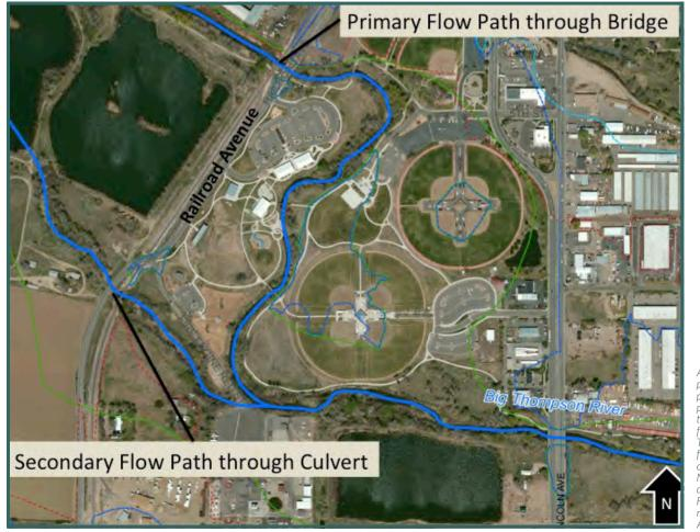
Aerial photo illustrating primary and secondary flow paths at Railroad Avenue. The primary flow path is through the bridge, and the secondary flow path is through a culvert. The flows along the secondary flow path are those that spill over into the River's Edge Natural Area upstream due to overtopping of Taft Avenue and First Street. The two flow paths merge downstream of Railroad Avenue in Fairgrounds Park.
