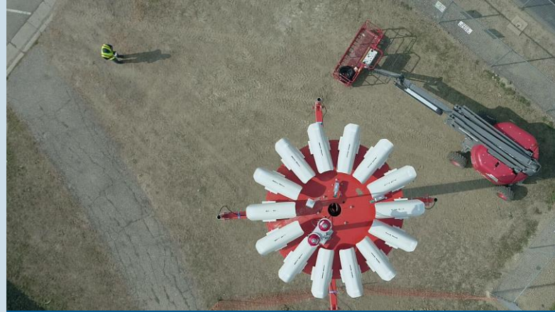
Remote tower camera mast aerial view (Source: CDOT)
