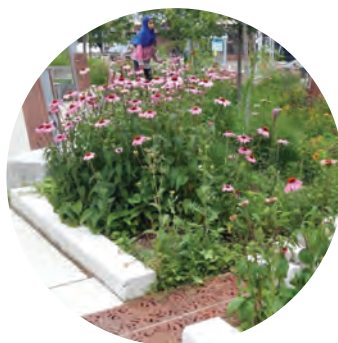
Rain gardens are ideal for smaller or residential systems to slow the movement of stormwater while collecting water to naturally water plants and vegetation.
