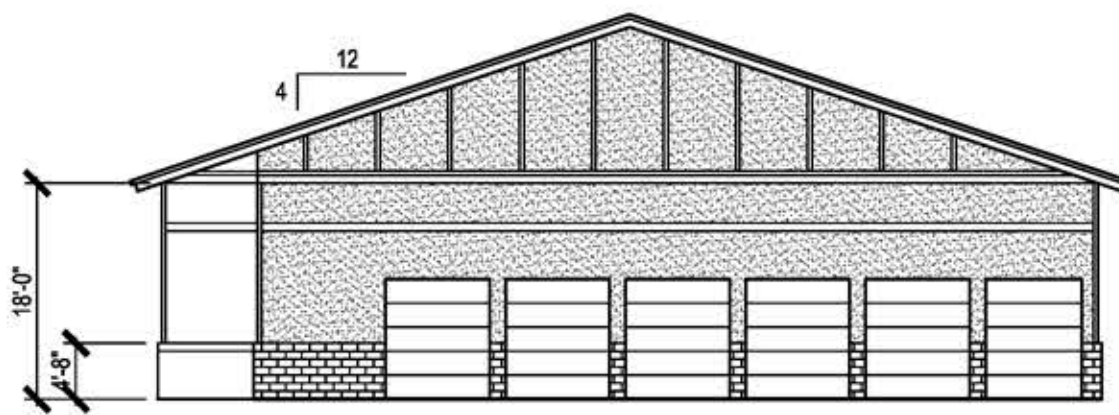
BUILDING C- NORTH ELEVATION 1/16"=1'-0"
