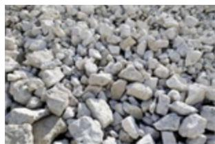
Due to erosion from waves to the banks of the reservoir it is necessary to install riprap along the banks of the reservoir. The riprap armoring will not only prevent nuisance erosion but also protect the bank of the reservoir from significant erosion that could threaten the structural integrity of the embankment.
