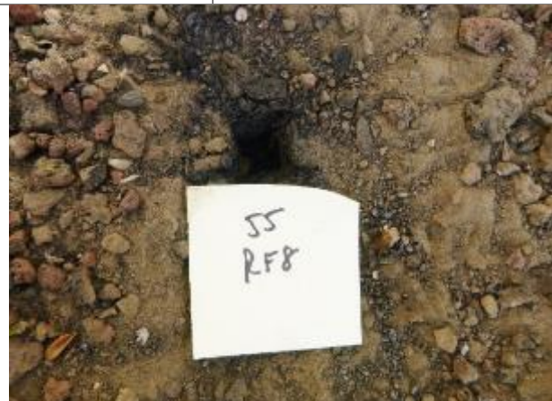
Photo #60 HA-55, black built-up asphaltic roofing with brown insulation
