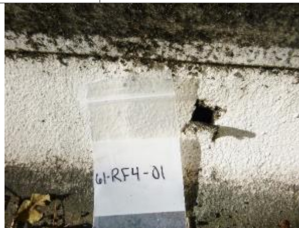
Photo #66 HA-61, white flashing with tan insulation and black tar
