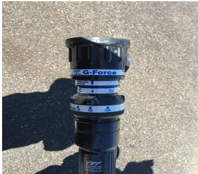
Figure 16: The nozzle is set to flow 500 LPM(130 GPM) and the pattern selector is adjusted all the way to the right.
