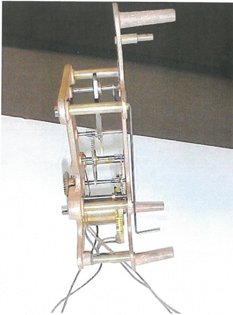
Below are photos showing the cast iron base and an original movement that has had a 1 rpm electric motor attached.
