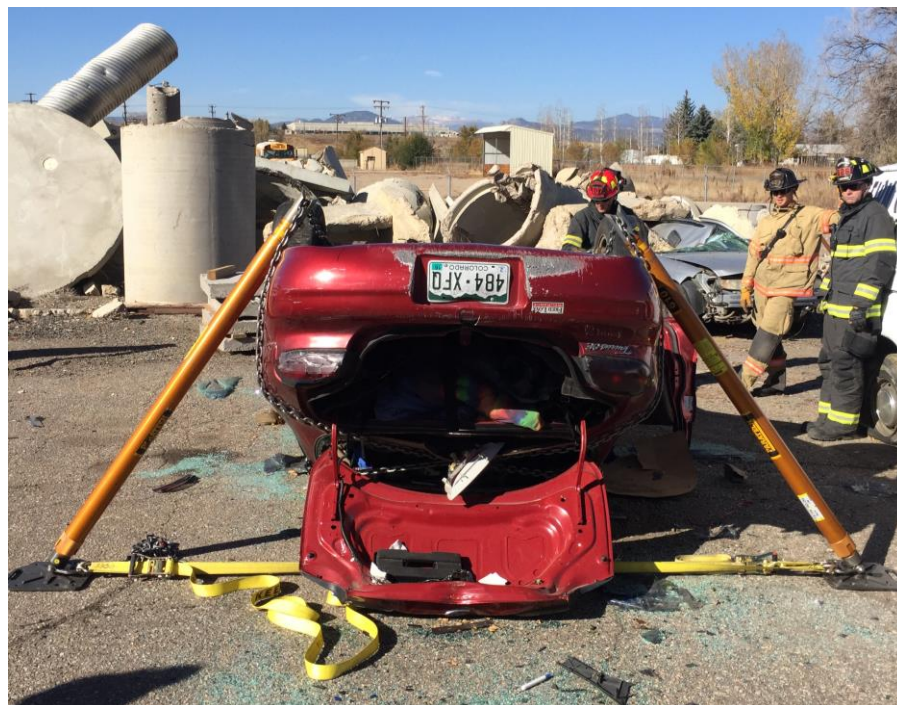
Figure 13 – Completed cradled stabilization
