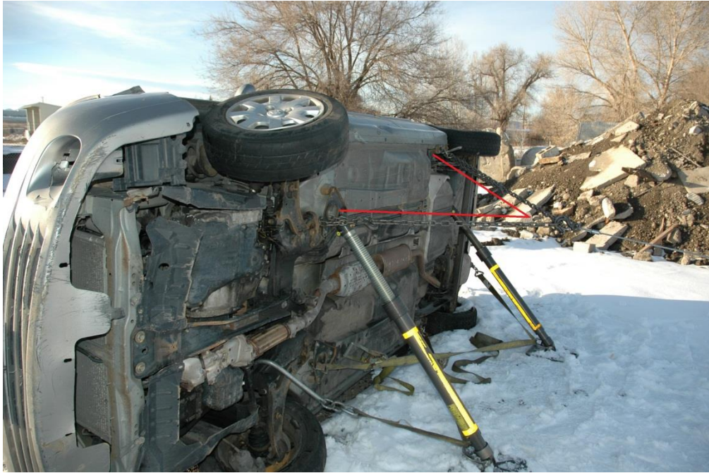
Figure 7 - Chain attached to the vehicle in a triangle formation
