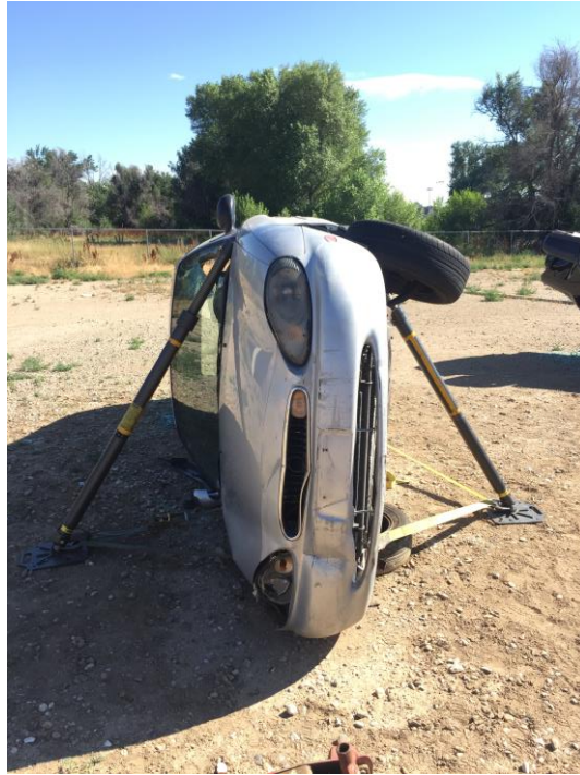
Figure 6 – Completed two-sided stabilization
