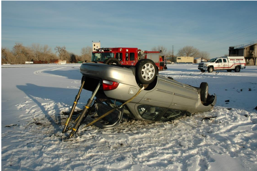
Figure 11 - Completed stabilization for a vehicle on its roof.
