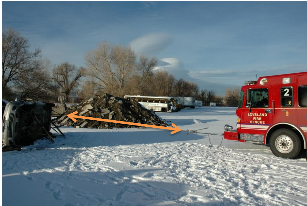
Figure 9 - Completed one-sided stabilization
