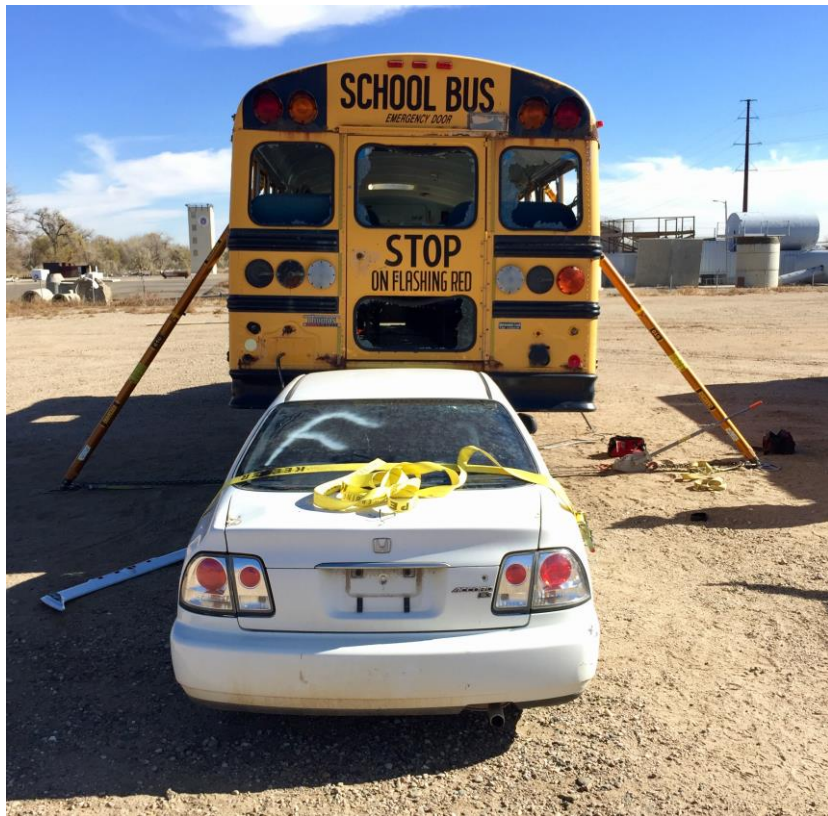
Figure 14 – Completed cradled stabilization
