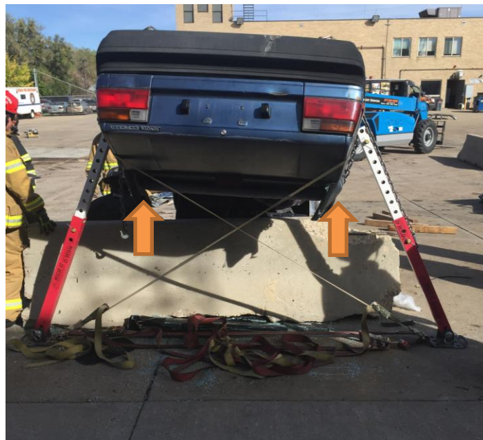
Figure 15 – Completed cradled stabilization with cross bracing
