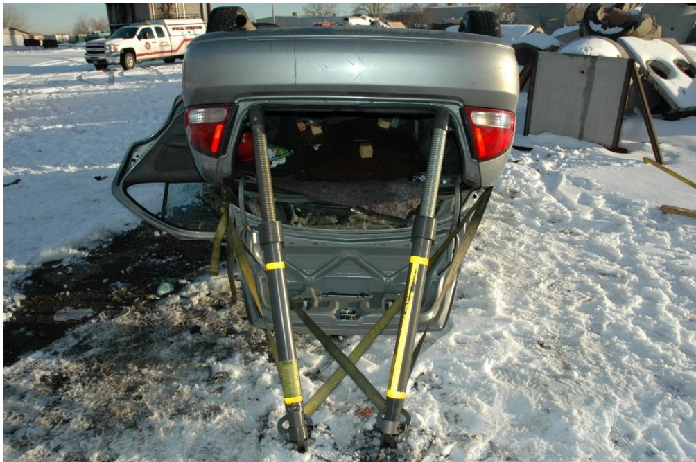
Figure 10 - Struts placed using the trunk opening for purchase points
