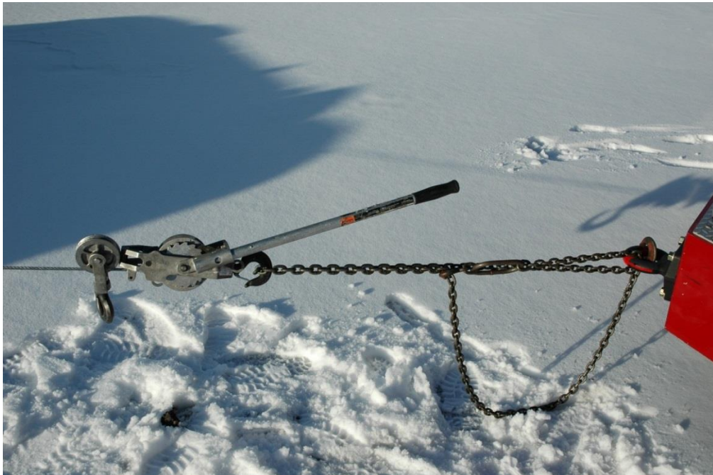
Figure 8 - Come Along secured to the vehicle
