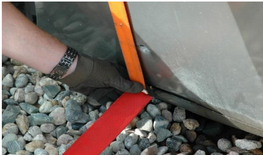
Figure 22 – Hook the strap at the bottom of the vehicle
