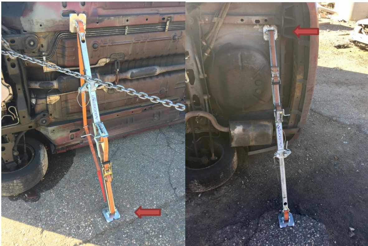
Figure 20 – The base of the strut can be placed at the bottom or the top
