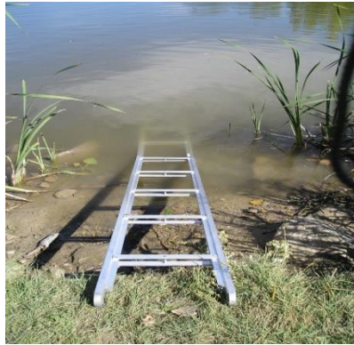
Figure 11.4 Driver/operators should take precautions so that intake strainers do not come in contact with the bottom of the water source.
