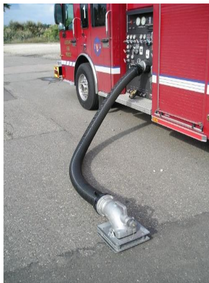
Hard suction hose and strainer secured tightly to intake.
