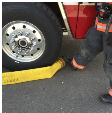
Fig.12 – FF pinning LDH to wheel.
