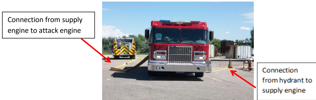
Fig. 18 – Water supply engine relay pumping to attack engine.
