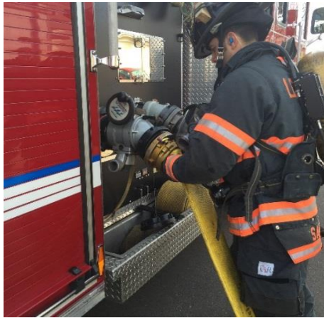
Fig. 14 – Making LDH connection.
