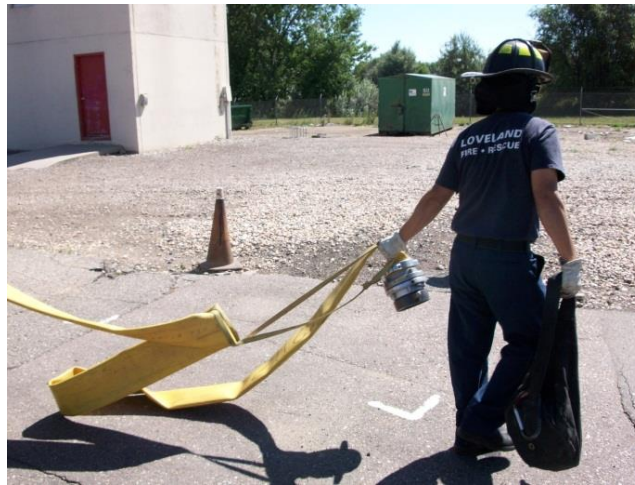
Fig. 2 – Deploying the LDH.
