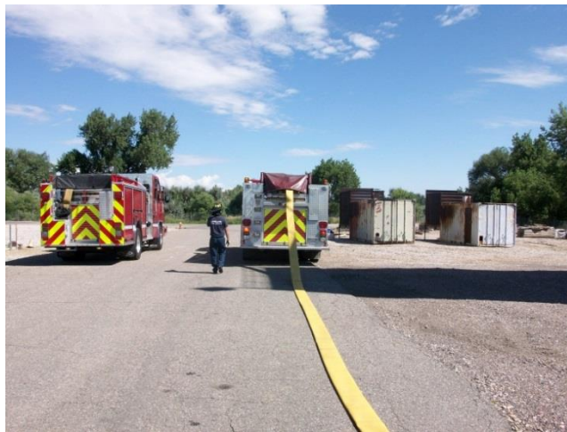
Fig. 5 – Engine deploying LDH.
