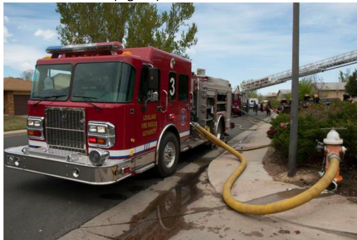
Fig. 19 – Relay pumping connection.
