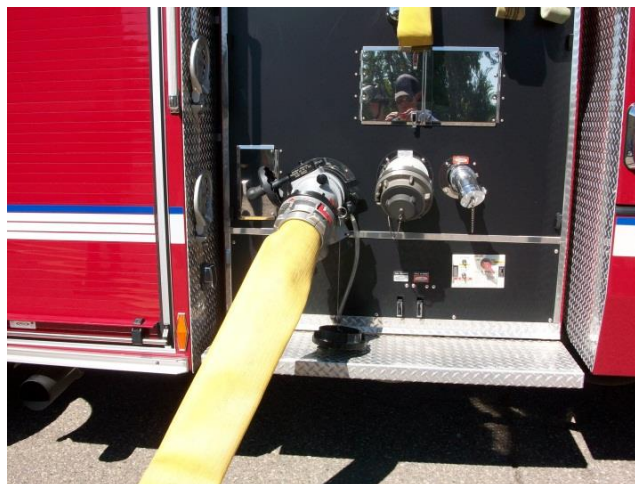
Fig. 7 – LDH connected to engine intake.
