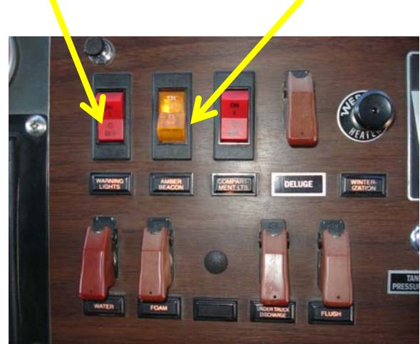
\*The amber beacon must be used at **all** times while on all non-active areas of the airport. The emergency lights must be used while responding to an emergency, on and off all airport property. This allows all air traffic to recognize that there is an emergency on the active or non-active areas of the airport.
