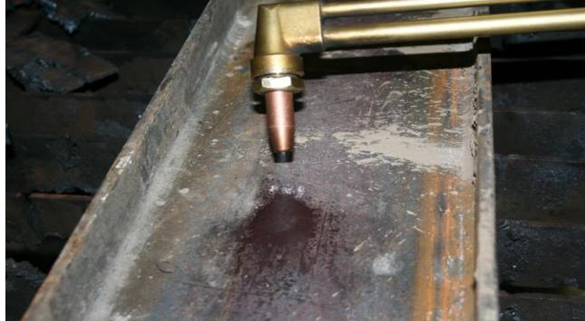
**Step 7:** Place the sparker directly in front of the tip and ignite the gasoline/oxygen mist.
