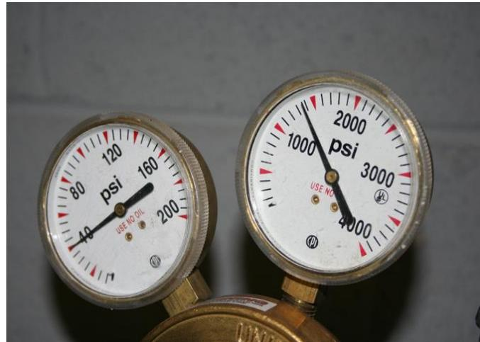
Notice that the gauge on the right indicates the total amount of pressure still in the cylinder, while the gauge on the left indicates the amount of pressure to the torch. Here the oxygen pressure is set to 40 psi. When opening the oxygen cylinder, always open the valve fully.
