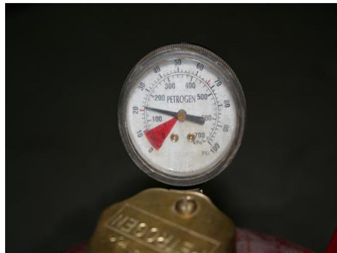
To insure good performance, keep the gasoline tank pressurized to 10-20 lbs. Here the gauge is set to 20 psi. Be sure to open the fuel valve fully when using this system.
