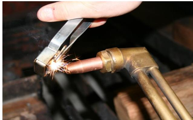
Avoid leaving the sparker in front of the tip too long before lighting, as the gasoline mist will soak the flint and you will have to wait for the wet flint to dry.
