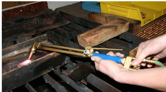
Touching the tip to the steel instantly brings the tip up to proper operating temperature.
