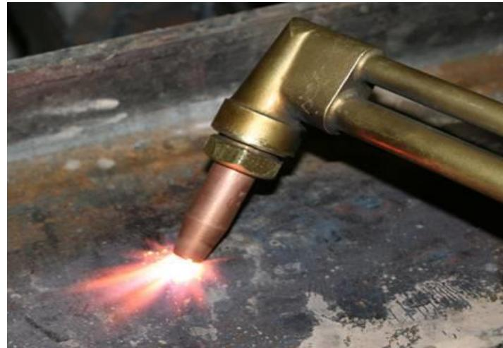
The flame is adjusted correctly when the steel is the hottest directly under the preheat flame. Some yellow/orange tint is acceptable, and should not alter performance.
