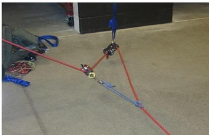
**Step 7:** Resting the haul system. Make sure that progress capture has grabbed the load. After progress capture is confirmed move the traveling pulley back to its beginning location by minding the prussic and walking back to the starting location.
