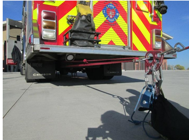
Anchor around axle with webbing
