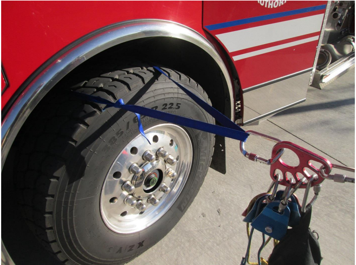
Webbing around axle and over tire- Advantage is higher tending stance.
