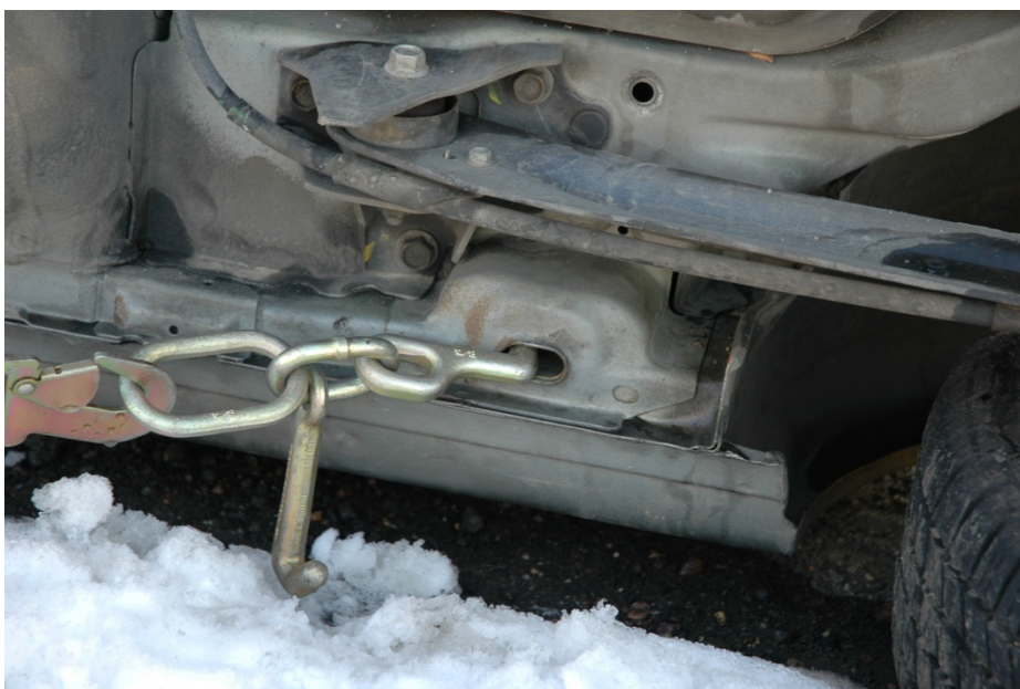
Figure 4 - Towman's clusters allow attachment to the unibody holes
