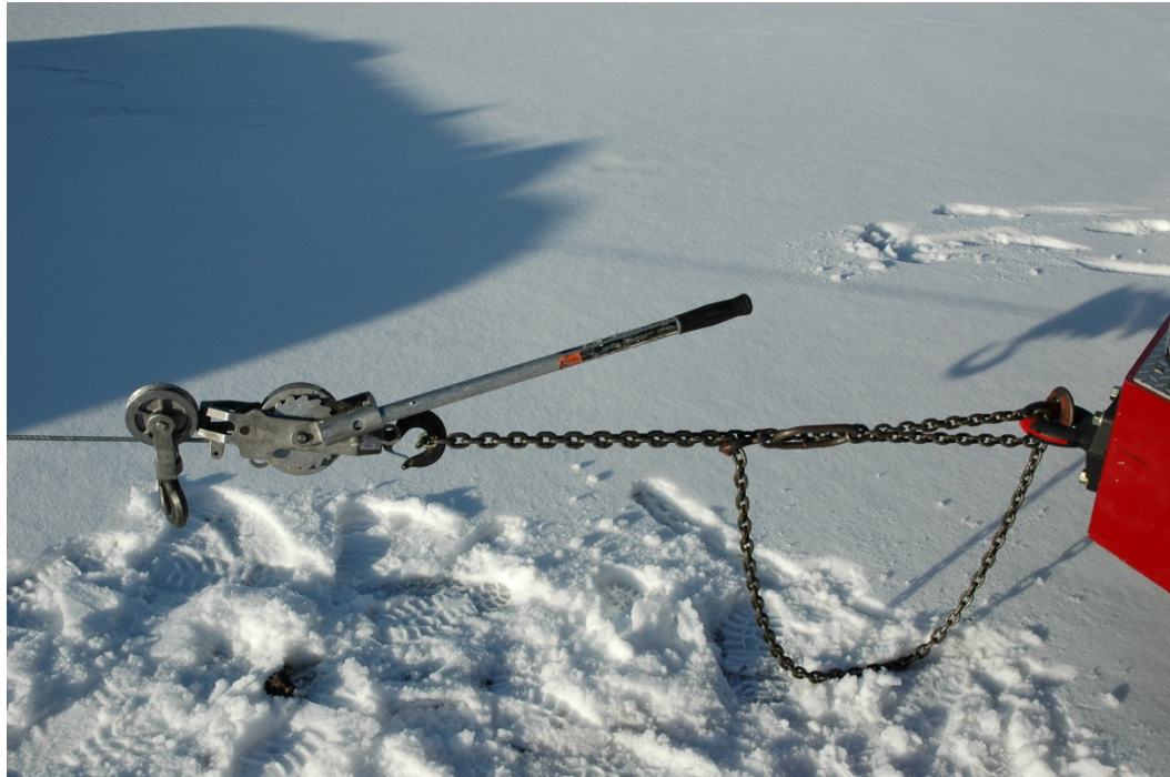
Figure 7 - Come Along secured to the vehicle
