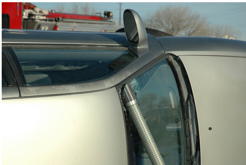
Figure 2 - Break glass to gain a purchase point if needed
