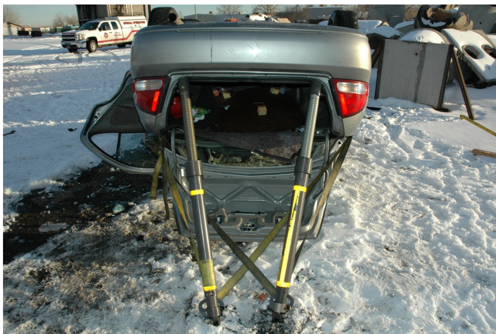
Figure 9 - Struts placed using the trunk opening for purchase points
