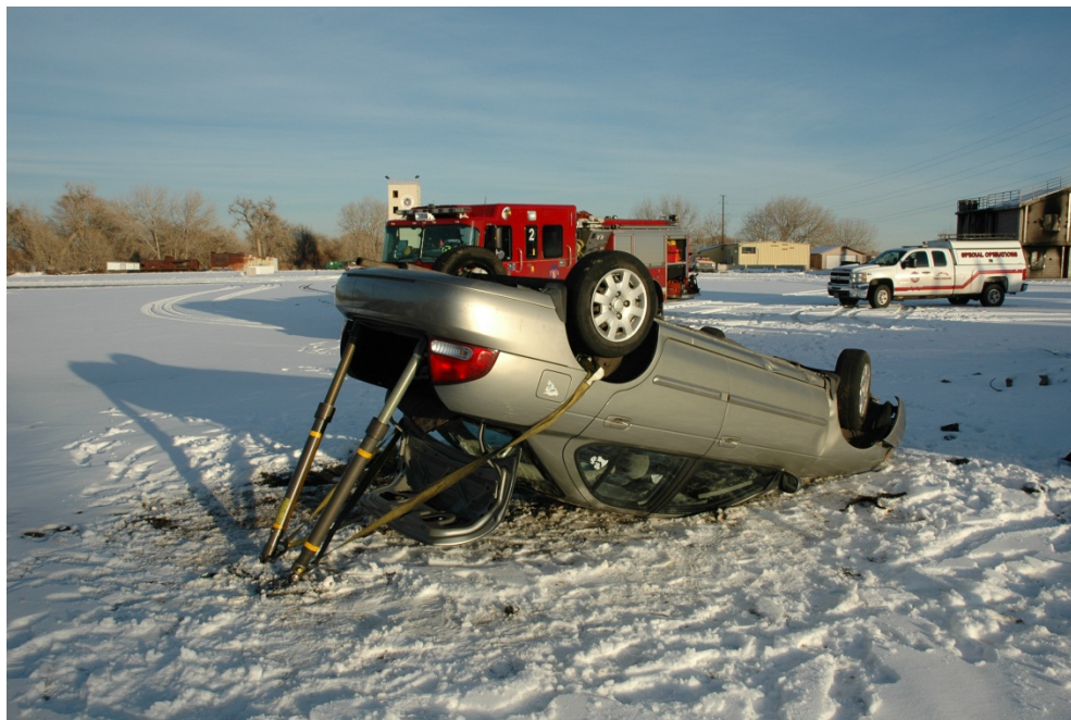
Figure 10 - Completed stabilization for a vehicle on its roof.
