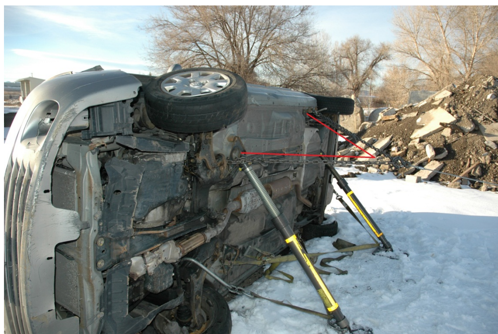
Figure 6 - Chain attached to the vehicle in a triangle formation
