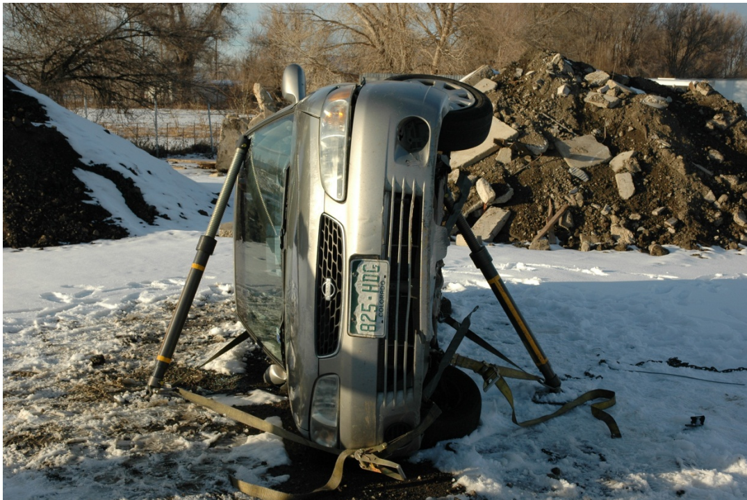
Figure 5 – Completed two sided stabilization
