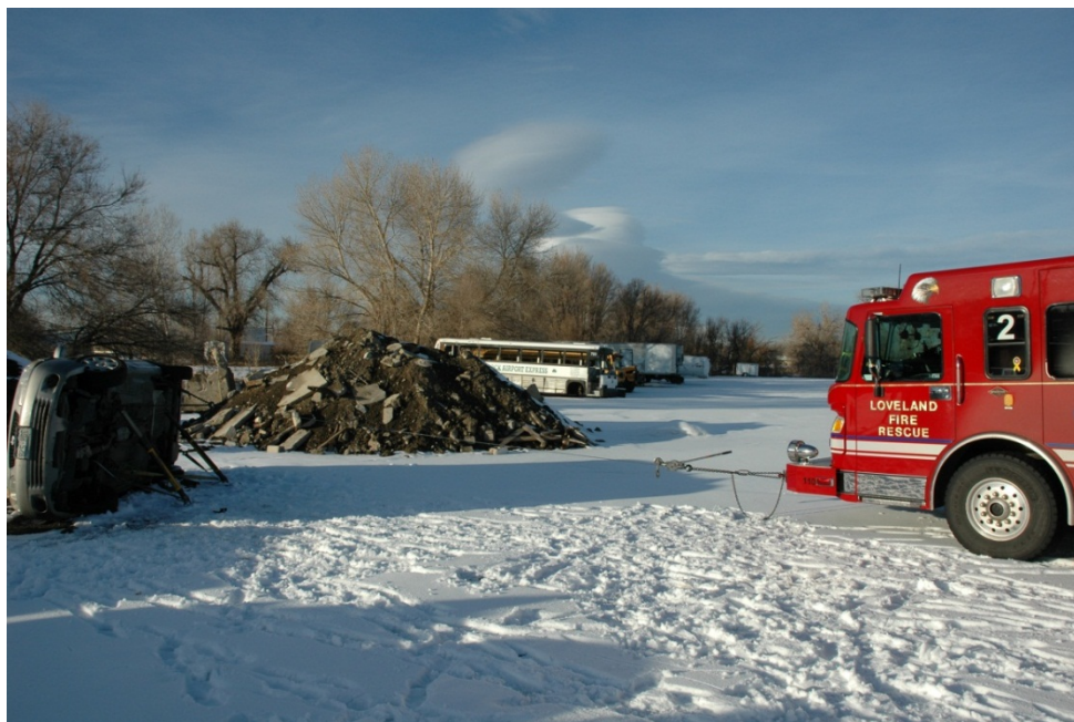
Figure 8 - Completed one-sided stabilization
