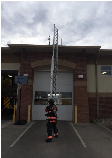
Figure 15, 16, 17 and 18: Rotating the ladder so the fly section is away from the building.
