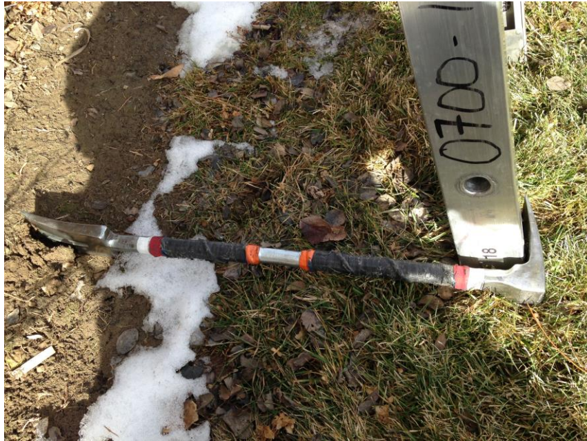
Figure 33: A halligan bar can be used to foot the ladder.
