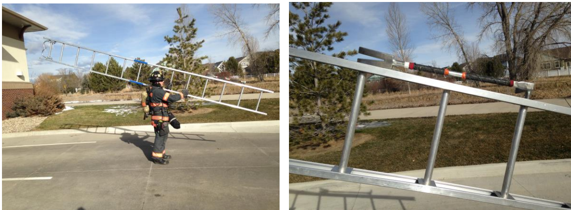
Figure 31 and 32: A halligan bar placed on the ladder beam for weight distribution.
