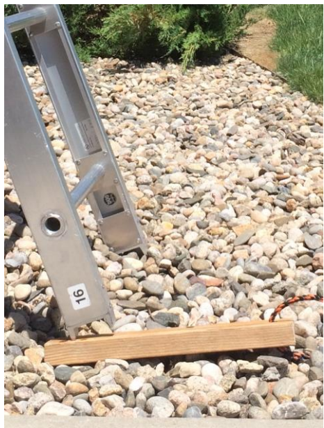
Figure 34 & Figure 35: Ladder chocks can be used to help level the ladder on uneven terrain or on a slope.
