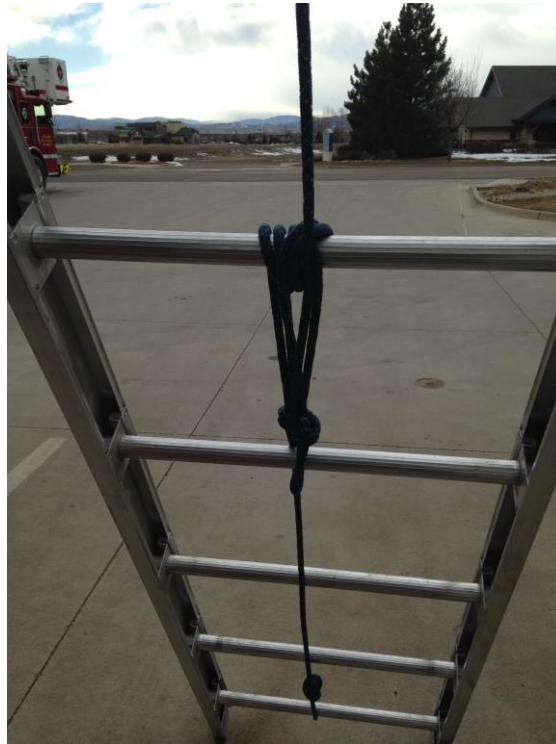
Figure 14: Tie off the halyard with a clove hitch and safety knot.
