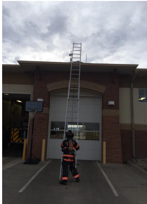
Figure 15, 16, 17 and 18: Rotating the ladder so the fly section is away from the building.
