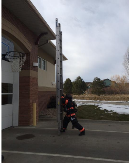
Figure 11: Use a controlled hand over hand motion to control the ladder extension.
