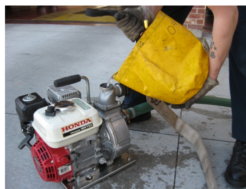
Fill pump casing completely with water prior to starting.
