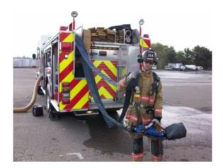
Once the location for the Blitz-Fire is selected by the officer, the legs of the unit must be folded into the operating position prior to charging the hose line. In most cases the unit does not need to be secured further, but in cases of a slippery surface such as loose gravel, snow, ice, and wet surface, it is imperative that the unit is secured properly prior to flowing water. The unit can be manned or unmanned and can be operated by a single firefighter.
