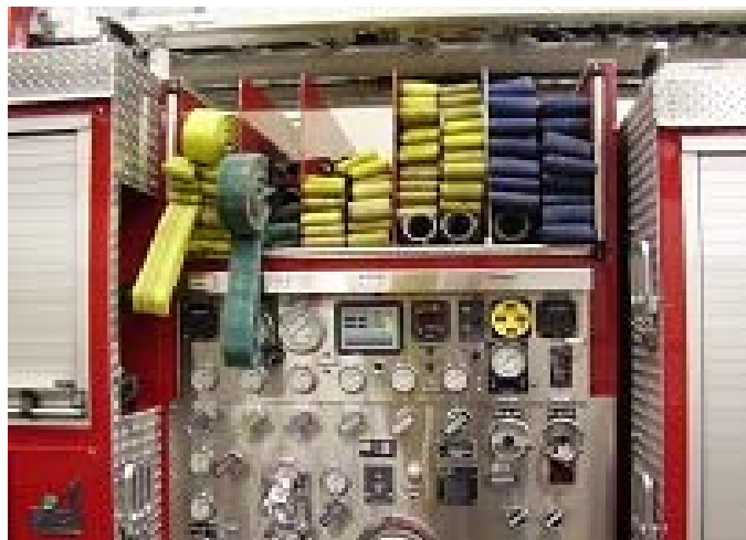
Figure 2 - Hose loads for a crosslay apparatus
