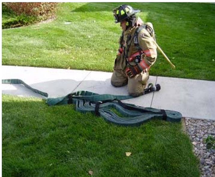
Figure 8 - The nozzle should be resting on top of the Gasner load prior to charging
