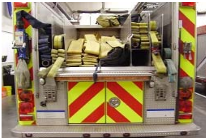
Figure 1 - Hose loads for a rear deploying apparatus
