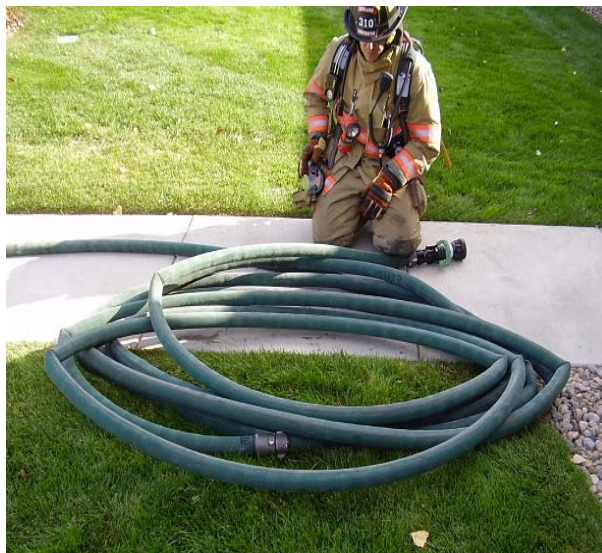
Figure 9 - Properly charged Gasner load
