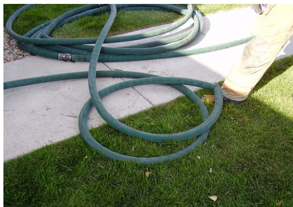
Figure 10 - Set up the loops based on the position of the nozzle person
