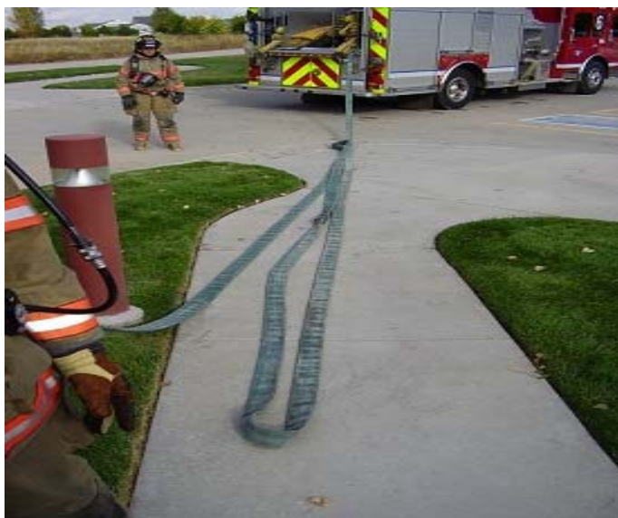
Figure 7 - Firefighter has cleared the hose bed
