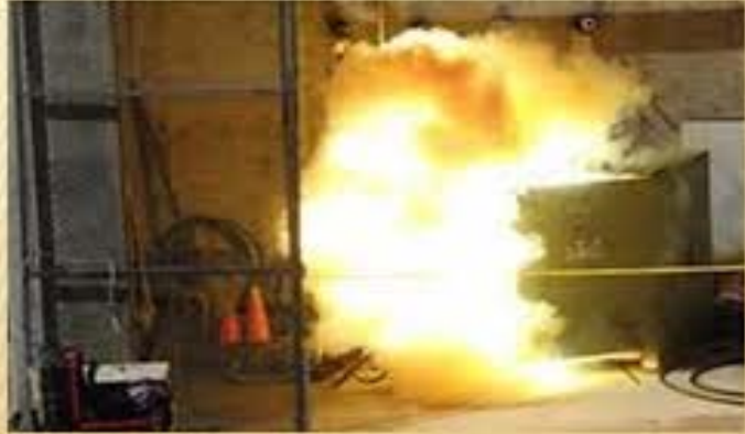
EXAMPLE OF ARC FLASH INCIDENT
