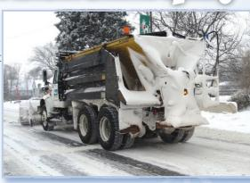
**Both ends working**When the snow falls, Loveland's dump trucks are equipped stem to stern to clear the roadways. On the front is a heavy duty snowplow and on the rear is a spreader for the de-icer loaded in the truck's
