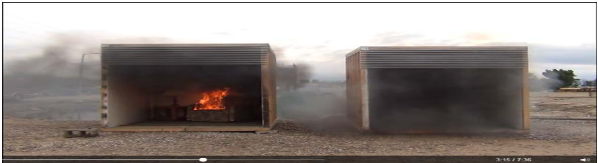
Fire Sprinkler activation in the right burn cell - 3:15 into fire demonstration.
