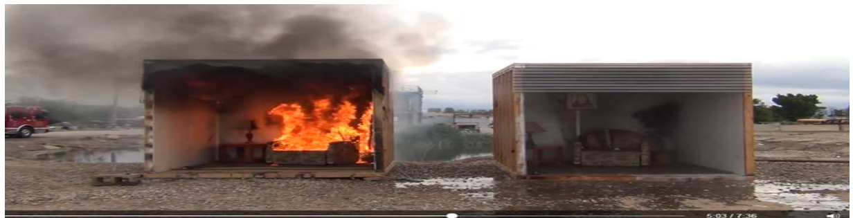
Fire in left burn cell at 5:03 – complete loss of all furnishings in the left cell and fire continuing to progress
