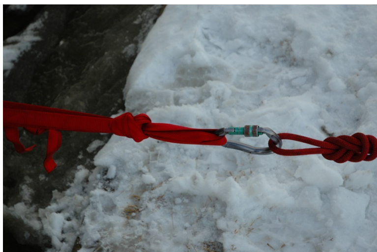
Figure 6 - Shortening the anchor strap
