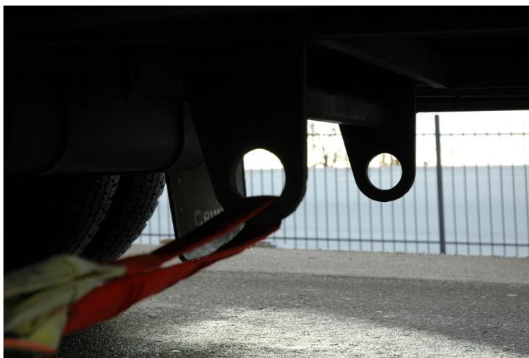
Figure 7 - Using the anchor point beneath the apparatus
