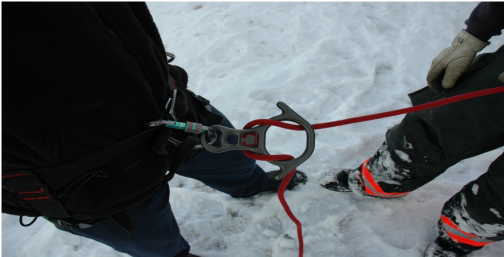
Figure 8: This rope is set up for the rescuer to use his right hand as the brake hand
