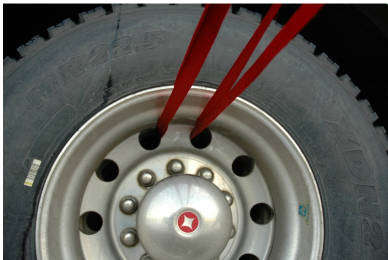
Figure 5 - Anchoring with webbing through the apparatus wheel.
