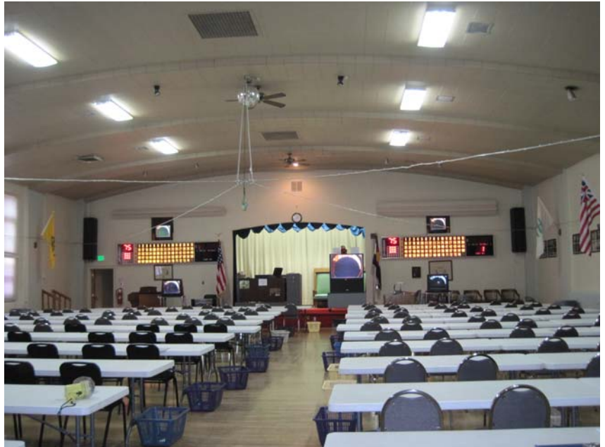
LEL7550 SECOND FLOOR LODGE ROOM AND STAGE, CAMERA FACING NORTH (NOTE ENGAGED PILASTERS ON EAST AND WEST WALLS AND RIBS ON CEILING, INDICATING STRUCTURAL TRUSS/FRAMING LOCATIONS)
